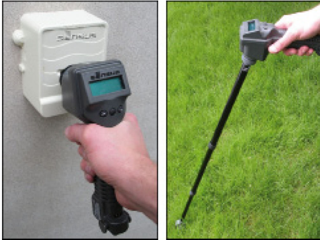
AutoGun touchgun or AutoGun with PitProbe extension can be used as a stand-alone unit for obtaining visual readings from Sensus encoders.
