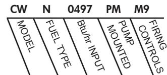
This heater is 495,000 Btu/hr natural gas Copper-Fin water heater. It is pump mounted and has F9 firing controls.
