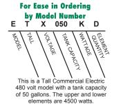
Notes: Water connections 3/4" NPT on all models. P.O.U. models available in single phase only. 6 gallon P.O.U. not available above 2500 watts or in 480 V. Non-simultaneous circuit only. Short & Tall models are factory wired for three phase service and are field converted to single phase.
