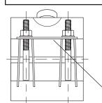
Stainless Steel Nuts and Studs - Type 304 stainless steel studs per ASTM A193 and A194. Heavy hex nuts are coated to prevent galling.
