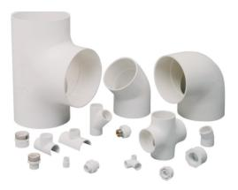
SPEARS<sup>®</sup> Schedule 40 PVC fitting designs combine years of proven experience with computer generated stress analysis to yield the optimum physical structure and performance for each fitting. Material reinforcement is uniformly placed in stress concentration areas for substantially improved pressure handling capability. Resulting products are subjected to numerous verification tests to assure the very best PVC fittings available.
