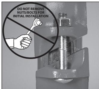
**1. DO NOT DISASSEMBLE THE COUPLING:** Style 009N/009H FireLock EZ™ Installation-Ready™ Rigid Couplings are designed so that the installer does not need to remove the bolts and nuts for installation. This design facilitates installation by allowing the installer to directly insert the grooved end of mating components into the coupling.
