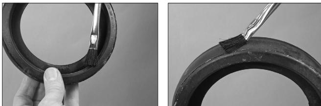
3. **FOR REASSEMBLY OF STYLE 009N/009H COUPLINGS, LUBRICATE GASKET:** Apply a thin coat of Victaulic Lubricant or silicone lubricant to the gasket sealing lips and exterior. It is normal for the gasket surface to have a hazy white appearance after it has been in service.
