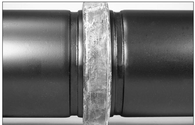
3. **JOIN MATING COMPONENTS:** Align the two grooved mating component ends. Insert the other mating component end into the gasket until it contacts the center leg of the gasket. **NOTE:** Verify that no portion of the gasket extends into the groove of either mating component.
