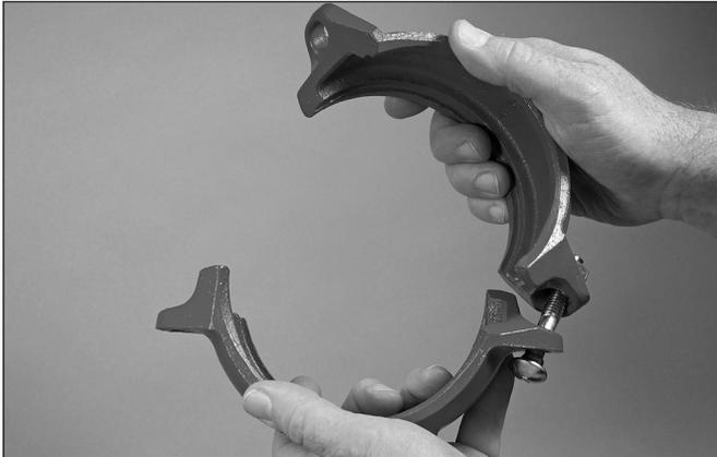
**4. TO FACILITATE REASSEMBLY:** One bolt can be inserted into the housings with the nut threaded loosely onto the bolt to allow for the “swing-over” feature, as shown above. **NOTE:** The nut should be backed off no further than flush with the end of the bolt.
