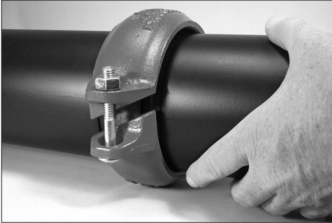
**4. ASSEMBLE JOINT:** Assemble the joint by inserting the grooved end of a mating component into each opening of the coupling. The ends of the grooved mating components shall be inserted into the coupling until contact with the center leg of the gasket occurs. A visual check is required to verify that the coupling keys align with the grooves in the mating components. **NOTE:** The coupling may be rotated to verify that the gasket is seated properly.
