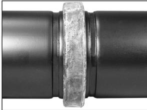
**3. JOIN MATING COMPONENTS:** Align the centerlines of the two grooved mating component ends. Insert the other mating component end into the gasket until it contacts the center leg of the gasket. **NOTE:** Verify that no portion of the gasket extends into the groove of either mating component.
