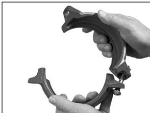
**4. TO FACILITATE REASSEMBLY:** One bolt can be inserted into the housings with the nut threaded loosely onto the bolt to allow for the “swing-over” feature, as shown. **NOTE:** The nut should be backed off no further than flush with the end of the bolt.
