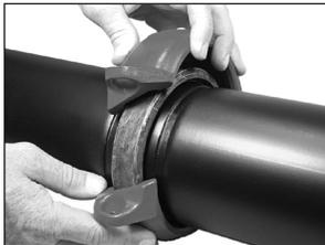
**5. INSTALL HOUSINGS:** Install the housings over the gasket. Verify that the housings’ keys engage the grooves completely on both mating components.
