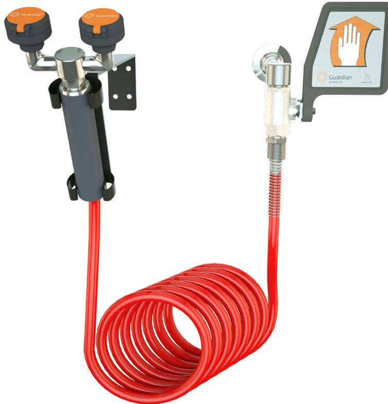
**Application:** Dual purpose eyewash/drench hose with ball valve and flag handle for wall mounting. Unit meets the provisions of ANSI Z358.1-2014 as both an eyewash and a drench hose. Unit may be left in the mounting bracket for use as a fixed eyewash, leaving user's hands free. Alternatively, unit may be removed for use as a drench hose to rinse any part of user's eyes, face or body. 12' nylon retractable hose coils to eliminate trip hazard.
