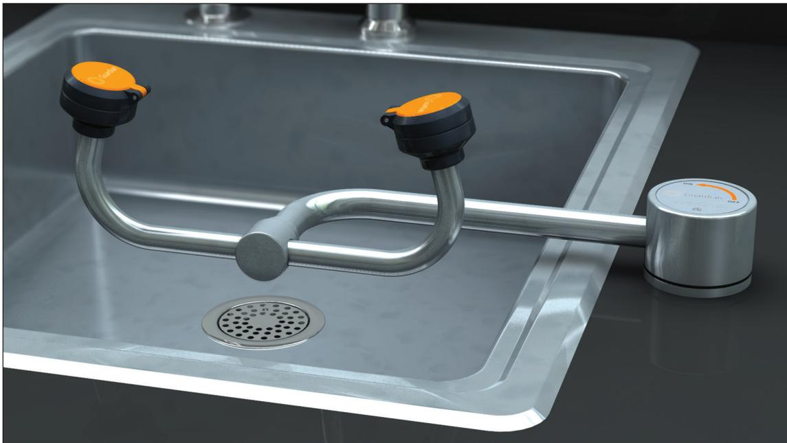
**Application:** All-stainless steel AutoFlow™ eyewash for mounting next to sink. Unit is constructed entirely in stainless steel. Ideal for use in highly corrosive environments, cleanrooms and pharmaceutical applications. Swinging the spray head assembly horizontally out over the sink activates the water flow. The unit remains in operation until the spray head assembly is swung back into the storage position, closing the valve.
