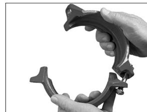
4. **TO FACILITATE REASSEMBLY:** One bolt can be inserted into the housings with the nut threaded loosely onto the bolt to allow for the “swing-over” feature, as shown. **NOTE:** The nut should be threaded no further than flush with the end of the bolt.
