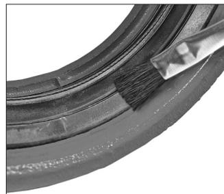
**3a.** If any conditions listed in the "NOTICE" on the following page are met, apply a thin coat of a compatible lubricant only to the gasket sealing lips. Refer to the "Lubricant Compatibility for Gaskets" table below.
