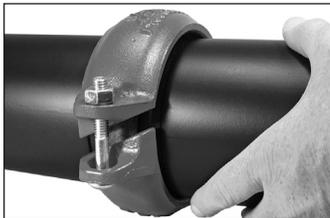
**4. ASSEMBLE JOINT:** Assemble the joint by inserting the grooved end of a mating component into each opening of the coupling. The grooved mating component ends shall be inserted into the coupling until contact with the center leg of the gasket occurs.
