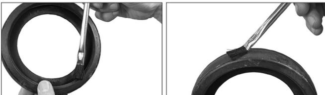
5. **FOR REASSEMBLY OF STYLE 009N COUPLINGS, LUBRICATE GASKET:** Apply a thin coat of a compatible lubricant to the gasket sealing lips and exterior. Refer to the “Lubricant Compatibility for Gaskets” table on page 1.
