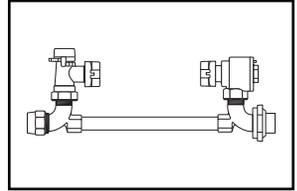
ANGLE KEY VALVE BY ANGLE DUAL CHECK VALVE
