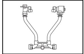
ANGLE KEY VALVE BY ANGLE DUAL CHECK VALVE (5/8" X 3/4" METER)
