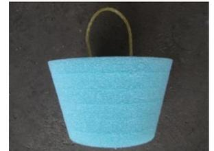
The DMplug is a non-pressure alternative for keeping debris and sediment from entering pipe and fittings. The tapered body allows for use in a variety of inside diameters. The DMplug will not absorb sediment or water. DMplugs can be made for a specific size for a custom fit.
