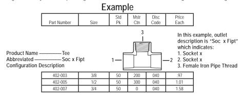
**Typical Valve Column Header** label identifies the following product particulars. Headers are generally preceded by identification of material type and configuration descriptions. Again, variations exist according to product type and configurations.
