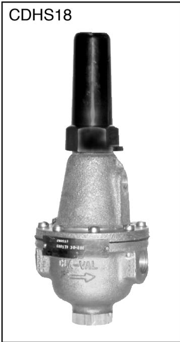
Normally Closed - Shifts to open on rise in sensed pressure
