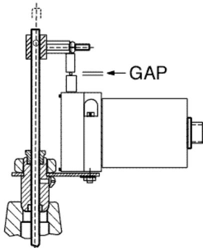
Coupler gap is set with valve in fully closed position. This establishes the minimum mechanical position for 4 mA output.
