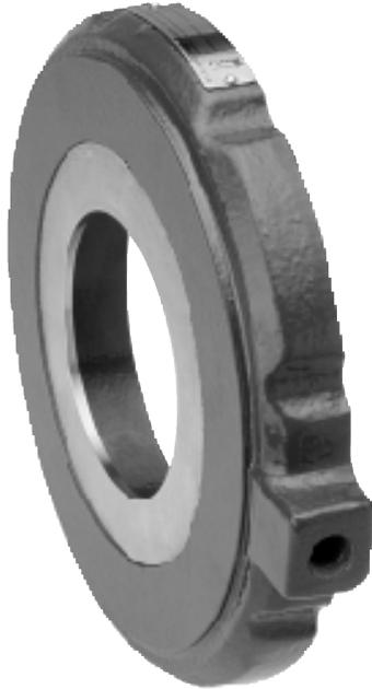
The Cla-Val Model X52E Orifice Plate Assembly is typically used with Cla-Val flow control valves. The orifice plate is an essential component used to generate a specific, predictable pressure drop in the system. The X52E uses a wafer design holder which offers a compact light-weight assembly that is easy to install. The X52E has a Chamfered "Inlet" side so even after installation, correct orientation can be easily verified.
