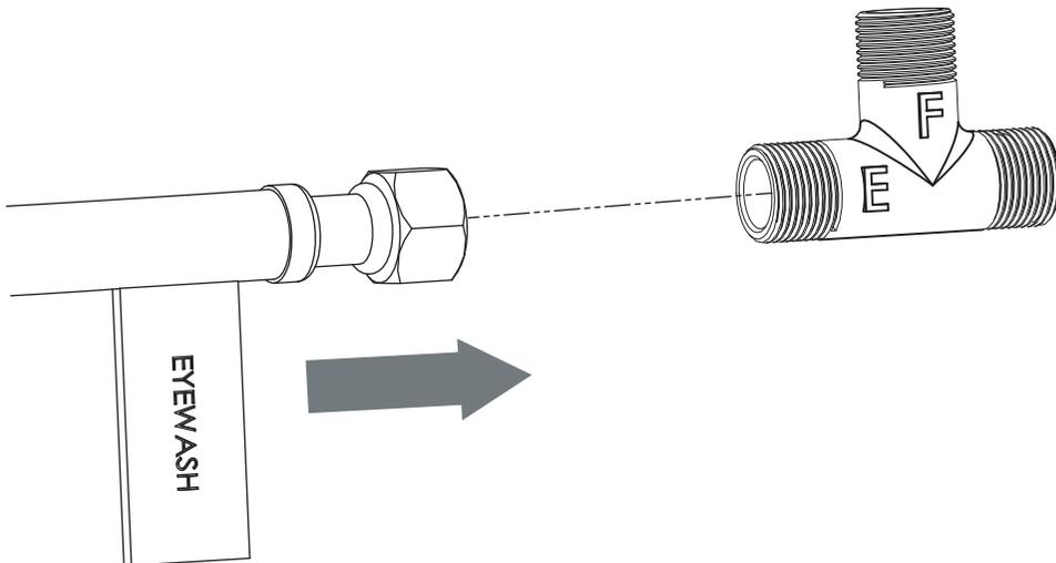
**CAUTION:** HOSES PROVIDED INCLUDE RUBBER COMPRESSION WASHERS FOR SEALING. DO NOT OVERTIGHTEN.
