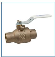
**Specifications UPC** Code 039923338532 Ball Valve Type S -- Female Solder Cup **Connection Type Stem Material** Silicon Bronze Valve Size 1/4 Material Lead Free Silicon Bronze **Valve Operator** CS Standard Lever Handle **Valve Operator Material** Metal - NIBCO - Steel - Zinc Plated S-585-80-LF 1/4 SOLDER FULL PORT BV **Description Turns/Operation** Quarter-Turn Weight 0.404 lb
