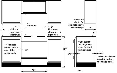
**Installation Information:** Before installing, consult installation instructions packed with product for current dimensional data.
