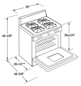
\*Dimension from wall to front of closed oven door. Dimension from wall to the front of closed oven door handle is 28-3/4". Minimum to cabinets on either side of the range
