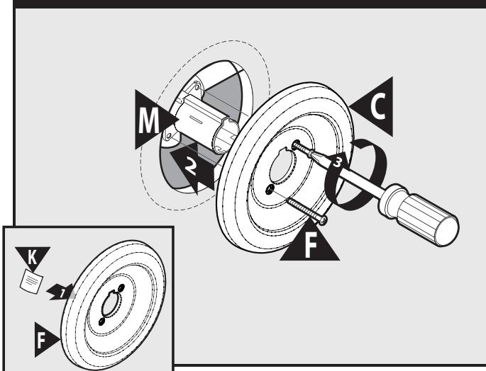
Place Product Identification Label (K) on back of Escutcheon. Use provided Escutcheon Screws (F) to secure the Escutcheon (C) to the wall. Slide Stop Tube (M) onto the existing valve.
