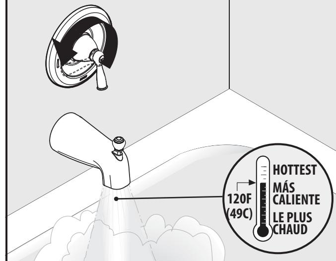
Rotate the lever counterclockwise until the water is to the maximum desired temperature, not to exceed 120 degrees F (49 degrees C). Seasonal maintenance of the maximum outlet temperature may be required due to changes in groundwater temperature. Turn lever to the off position once the temperature is set.
