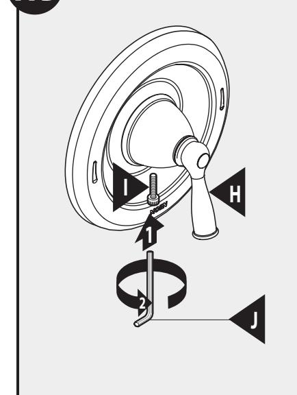
Using 7/64 inches hex wrench (J), insert and tighten hex screw (I) into lever (H).
