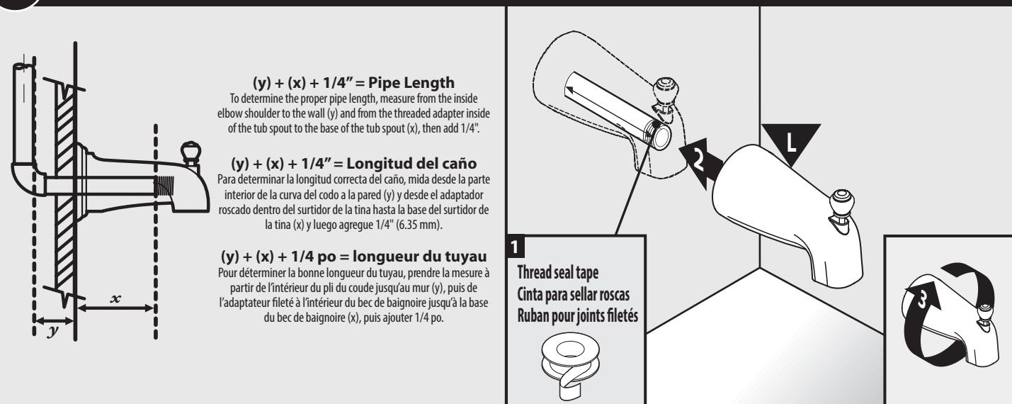
IPS (threaded) spouts are designed to screw onto a pipe with 1/2" male pipe threads. An IPS threaded adapter may be necessary (not included). To determine the proper pipe length, measure from the inside elbow shoulder to the wall (y) and from the threaded adapter inside of the tub spout to the base of the tub spout (x), then add 1/4". Place thread seal tape around the pipe threading and a sealant (plumbers putty or caulk) around the base of the pipe to prevent leaking behind the wall.
