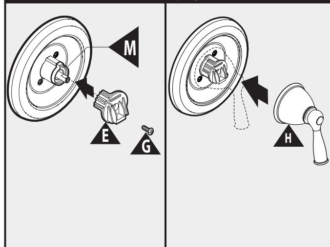
Attach plastic handle adapter (E) to the cartridge stem using the 1/2" adapter screw (G). Make sure the ridges on the back of the adapter (E) are to the left of the tab on limit stop (M). Place the lever (H) on the lever handle adapter.
