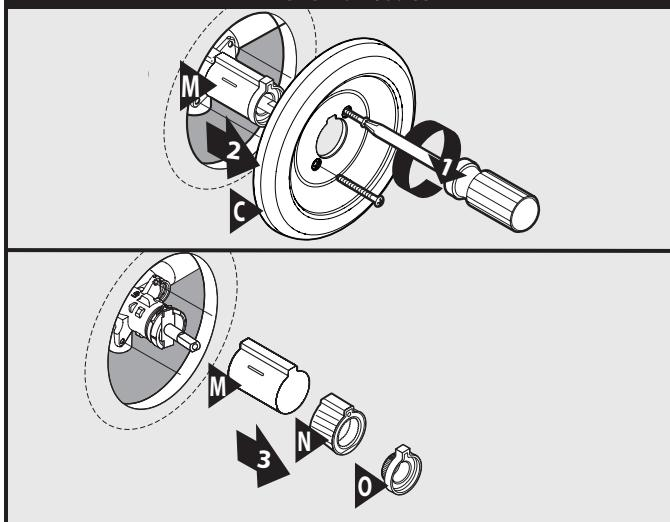
To remove the escutcheon (C) (cover plate) unscrew the two screws counterclockwise with a Phillips screwdriver. After removing the two screws, pull off the escutcheon plate from the valve and remove the stop tube (M), key stop (N) and adjustable temperature limit stop (O).
