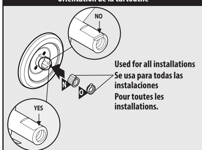
Rotate so the notch at the end of the stem is facing down towards the drain. Insert the key stop (O) and the adjustable temperature limit stop (N) into stop tube as shown.
