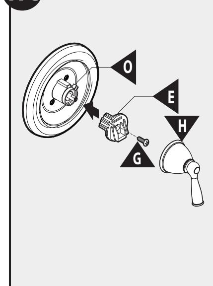
After setting the adjustable temperature limit stop to the desired position, remove the lever (H), reattach the lever handle adapter (E), adapter screw (G), and lever (H) – make sure ridges on back of (E) are to the left of the tab on (O).
