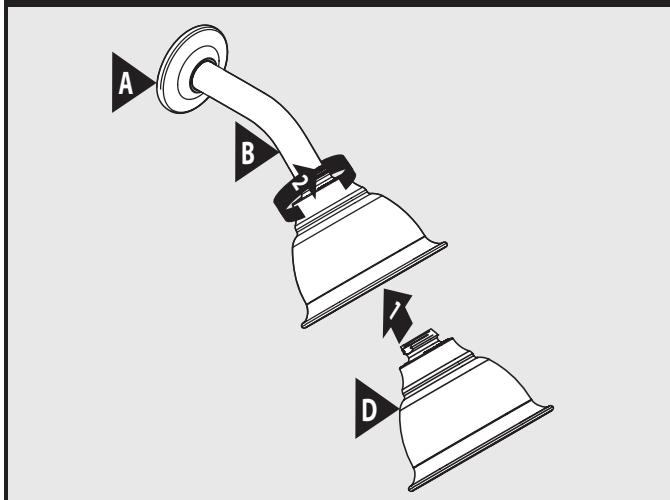
If there is a rubber washer inside the threaded adapter on the showerhead, thread the showerhead onto the shower arm as shown above. If there is no rubber washer in the showerhead, proceed to step 7A.
