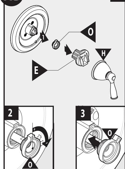
Remove the lever (H) and lever handle adapter (E). Note the position of the stop. Position the adjustable temperature limit stop (O) so the lever tops at that position. This prevents the lever from being turned into an unsafe temperature.
