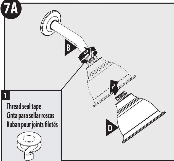
Wrap thread seal tape around threads at bottom of shower arm (B). Remove any debris from the shower arm to ensure proper flow. Thread showerhead (D) onto shower arm (B). Tighten with wrench.
