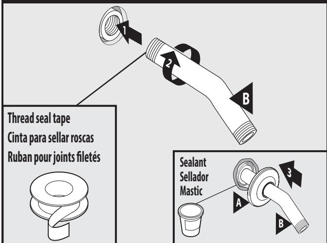
Wrap thread seal tape around the threads of the shower arm (B) then screw the arm into the threaded connection in the wall. Seal around shower arm hole with sealant (caulk) then slide Shower Arm Flange (A) over Shower Arm (B).
