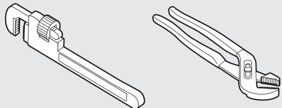
Unscrew the shower arm by hand and remove the flange. A pipe wrench or pliers might be required.
