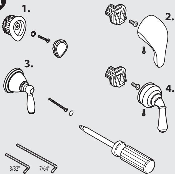
The knob 1 and lever 3 require a Phillips screwdriver for removal. Levers 2 and 4 require a 7/64" hex wrench (included) along with a Phillips screwdriver. Some models may require a 3/32" hex wrench (not included).
