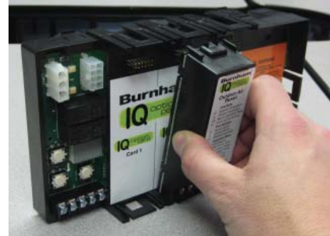
Insert IQ Option Card into selected slot
