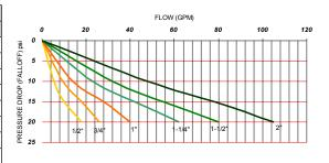
Note: Flow curves are based on static conditions of 100psi inlet pressure and 50 psi outlet pressure.
