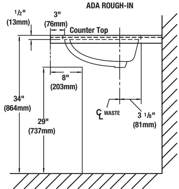
Note: All dimensions and specifications are nominal and may vary; Dimensions of 8" and greater have a tolerance of +3%. Dimensions less than 8" have a tolerance of +5%.
