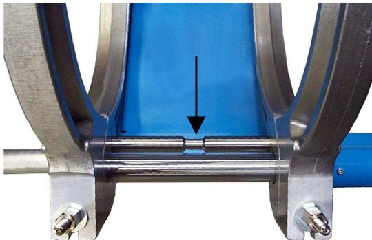
There is a tear-off bar mounted between the movable and the fixed clamping shells on the basic machine. It prevents the heating element from sticking to the heated-up pipe ends.
