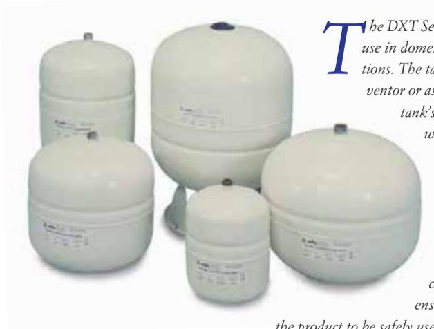
**T**he DXT Series diaphragm thermal expansion tank is designed for use in domestic system installations for sanitary hot water applications. The tank is installed in systems equipped with a backflow preventor or as an add-on to direct or indirect water heaters. The tank's function is to absorb the increased volume of water which results from the heating process, thereby keeping the system's pressure below the relief valve settings.
