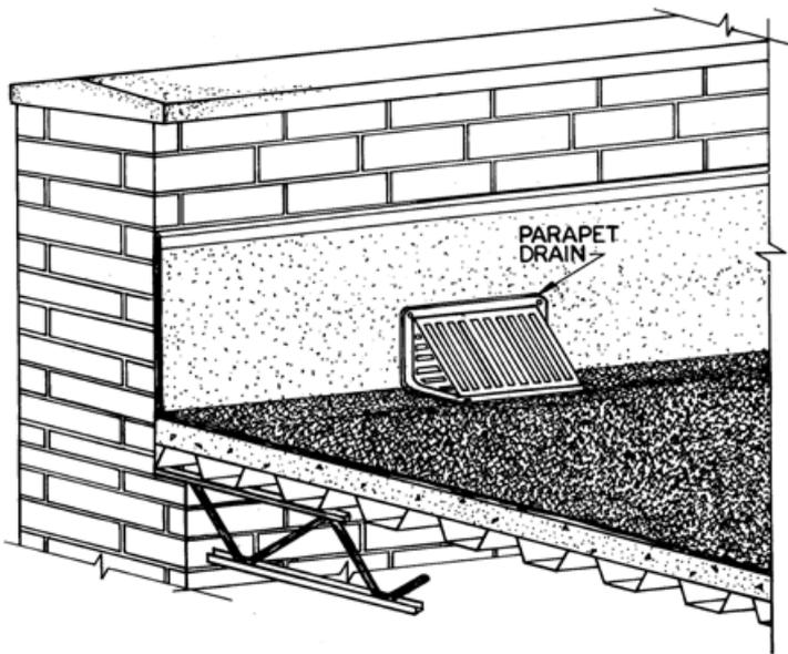
24700 Parapet Overflow Drain
