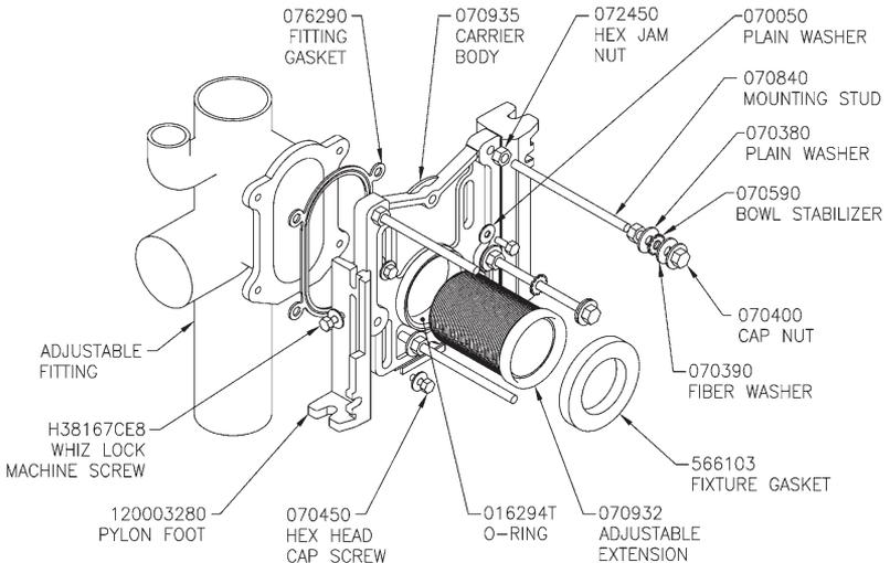
**SPECIFICATION:** JOSAM 12000-OR Series coated cast iron CHASE-SAVER® II Closet Carrier with adjustable connection, adjustable pylon feet, ABS extension with integral test cap, chrome plated trim, coated accessories and JIFFEE-SEAL Neoprene fixture gasket, for use with blowout or siphon jet water closets.
