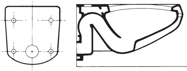
This type, because of its quiet, efficient, sanitary flushing action, is usually specified in most commercial, institutional and hotel applications. Water is introduced into the bowl through the rim and up leg of trap through jets placed there to fill the trapway thus creating siphonic action to quickly evacuate the bowl. The large water surface in the bowl insures sanitation.
