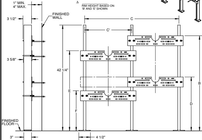
RECOMMEND ALL FEET BE SECURED TO FLOOR WITH 1/2" BOLTS AND ANCHORS BY OTHERS
