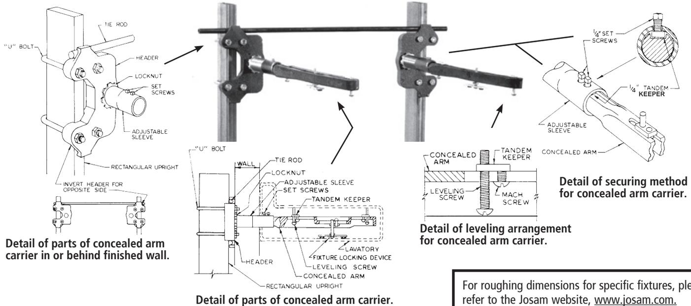
**Detail of parts of concealed arm carrier in or behind finished wall.**
