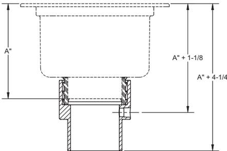
DIMENSION A = HEIGHT OF DRAIN BODY
