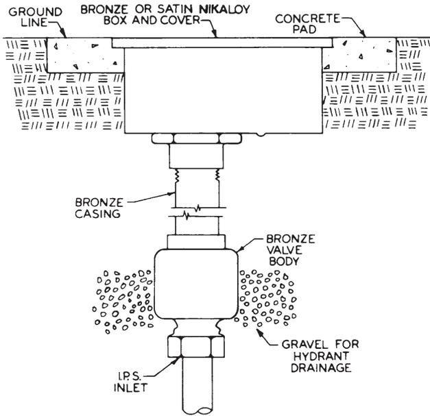
71600 Series Hydrant shown installed in a yard
