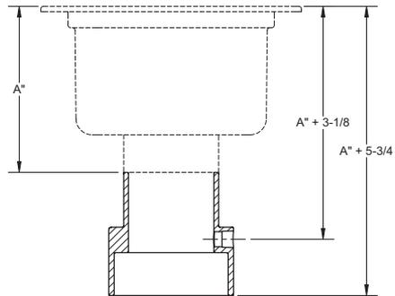
DIMENSION A = HEIGHT OF DRAIN BODY
