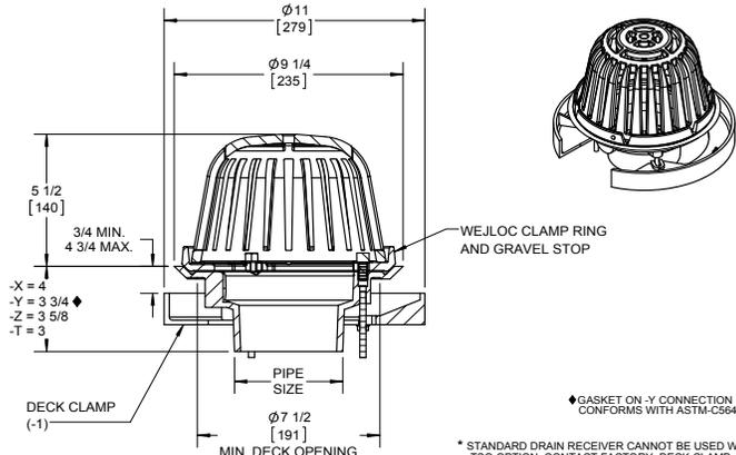
\* STANDARD DRAIN RECEIVER CANNOT BE USED WITH -TSO OPTION. CONTACT FACTORY. DECK CLAMP CANNOT BE USED WITH -TSO OPTION IN 4" SIZE.
