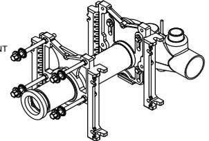
▲ FOR DIMENSION SHORTER THAN 5-1/2" (1" MIN) CUT EXTENSION FOR LONGER EXTENSION (10-1/2" MAX) SPECIFY (-10).
