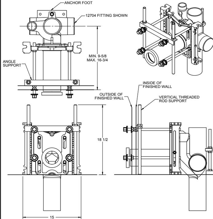
RECOMMEND CONCRETE ANCHORS WITH 750 LBS. PULL-OUT FORCE EACH.
