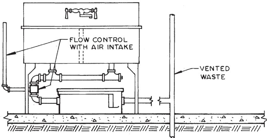
60115A Series Interceptor installed on floor under sink.
