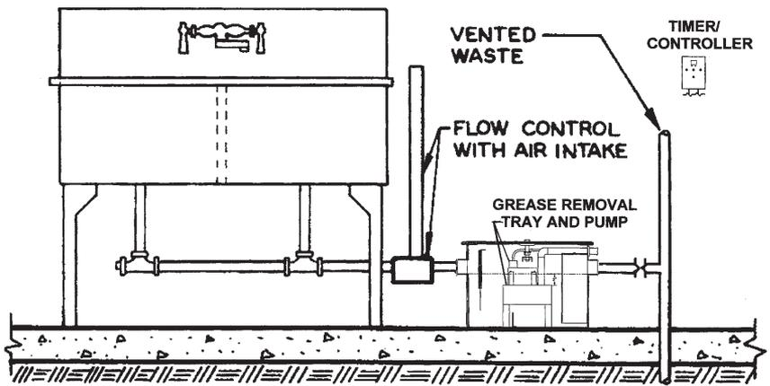
60100H-GRD Series Interceptor on floor, servicing a sink, shown installed with an optional -GRD Grease Removal Device.
