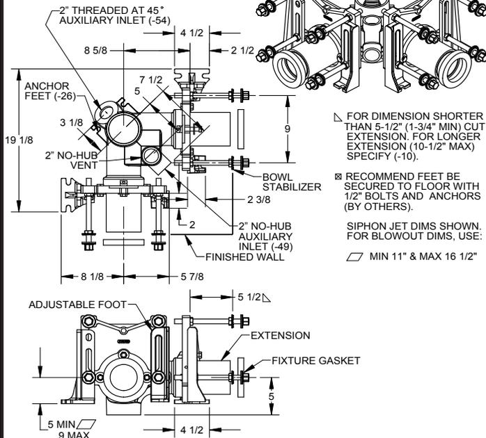
△ FOR DIMENSION SHORTER THAN 5-1/2" (1-3/4" MIN) CUT EXTENSION. FOR LONGER EXTENSION (10-1/2" MAX) SPECIFY (-10).
