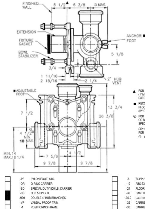
▲ FOR DIMENSION SHORTER THAN 5-1/2" (1" MIN) CUT EXTENSION. FOR LONGER EXTENSION (10-1/2" MAX) SPECIFY (-10)
