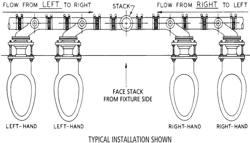
1. If flow in waste line is **from the right of the stack**, the closet fitting should be a **right-hand fitting**.
