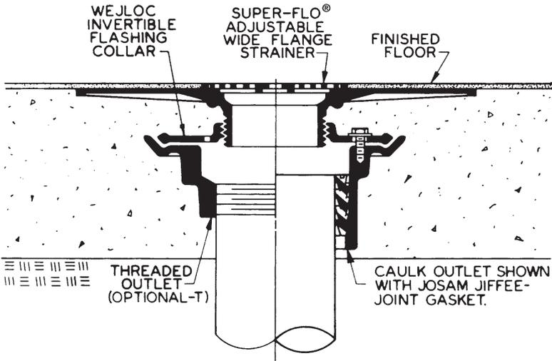
3000-WF6S Series SUPER-FLO® Adjustable Strainer Floor Drain shown installed in a composition deck floor. Wide flange assures that bonding of floor material is watertight and permanent.
