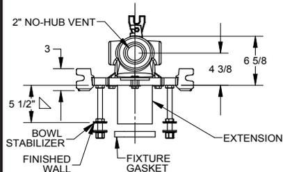
△ FOR DIMENSION SHORTER THAN 5-1/2" (1" MIN) CUT EXTENSION FOR LONGER EXTENSION (10-1/2" MAX) SPECIFY (-10).
