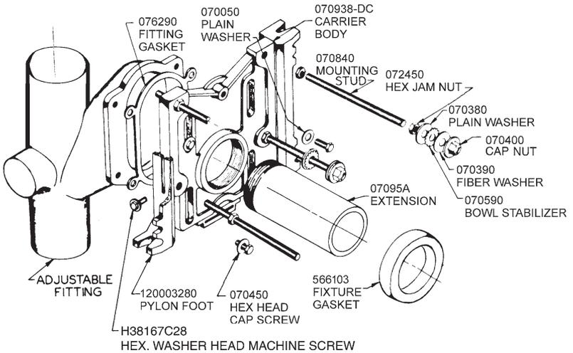
**SPECIFICATION:** JOSAM 12000-PF Series coated cast iron CHASE-SAVER® II Closet Carrier with adjustable connection, adjustable pylon feet, ABS extension with integral test cap, chrome plated trim, coated accessories and JIFFEE-SEAL Neoprene fixture gasket, for use with blowout or siphon jet water closets.
