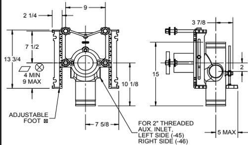
∇ FOR DIMENSION SHORTER THAN 5-1/2" (1" MIN) CUT EXTENSION FOR LONGER EXTENSION (10-1/2" MAX) SPECIFY (-10).
