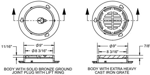
BODY WITH SOLID BRONZE GROUND JOINT PLUG WITH LIFT RING
