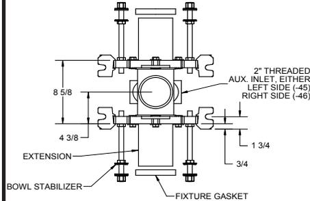
∇ FOR DIMENSION SHORTER THAN 5-1/2" (1" MIN) CUT EXTENSION FOR LONGER EXTENSION (10-1/2" MAX) SPECIFY (-10).
