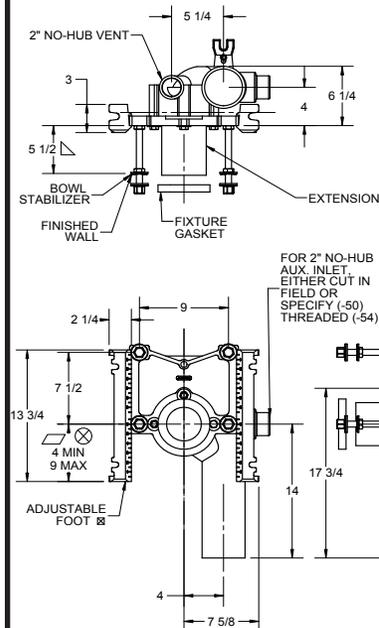
FOR 2" NO-HUB AUX. INLET EITHER CUT IN FIELD OR SPECIFY (-50) THREADED (-54)
