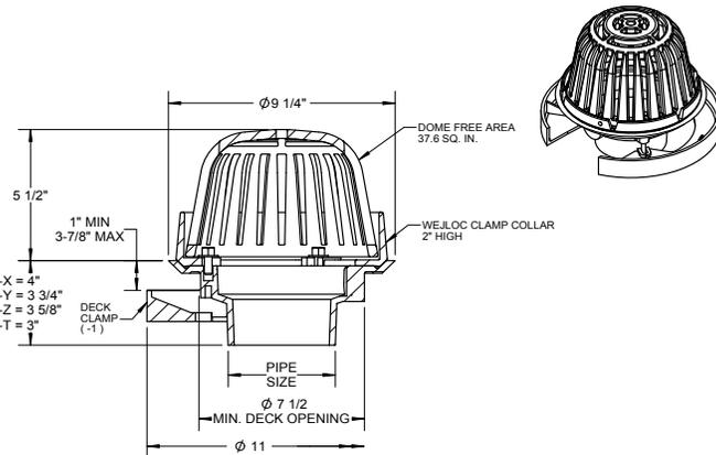
● GASKET ON -Y CONNECTION CONFORMS WITH ASTM-C564
