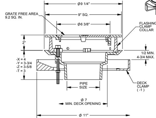
\* -TSO BODY CANNOT BE USED WITH DRAIN RECEIVER (-2, -3 & -3C)
