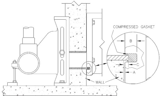
**For closets which have a groove with a rectangular cross-section, use this formula:**  $C = A + B - 1/2''$
