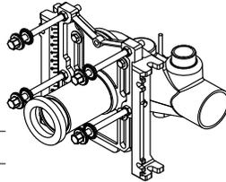
∇ FOR DIMENSION SHORTER THAN 5-1/2" (1" MIN) CUT EXTENSION FOR LONGER EXTENSION (10-1/2" MAX) SPECIFY (-10).
