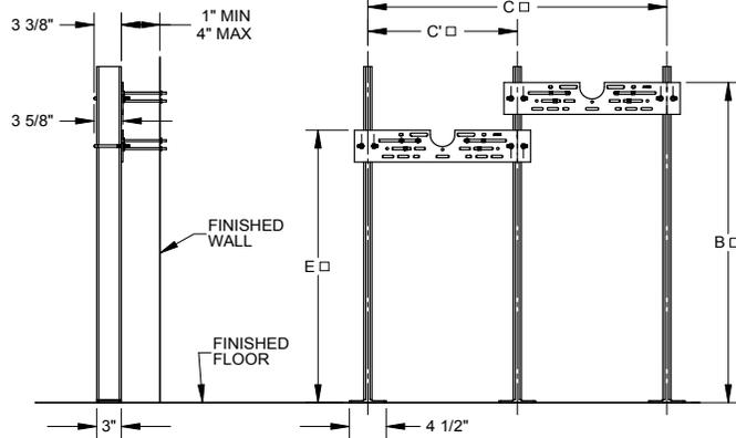
RECOMMEND ALL FEET BE SECURED TO FLOOR WITH 1/2" BOLTS AND ANCHORS BY OTHERS.
