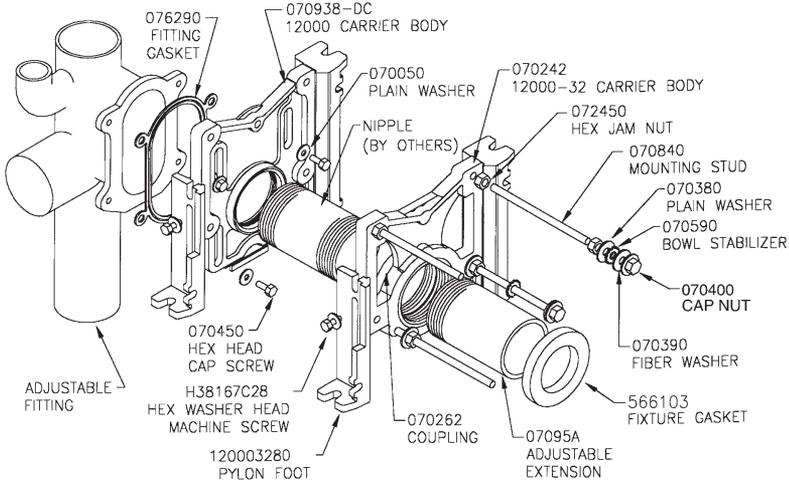
**SPECIFICATION:** JOSAM -32 coated cast iron Wide Chase Closet Carrier with adjustable closet connection, adjustable pylon feet, ABS extension with integral test cap, chrome plated trim, coated accessories and JIFFEE-SEAL Neoprene fixture gasket, for use with blowout or siphon jet water closets.
