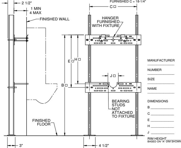
RECOMMEND ALL FEET BE SECURED TO FLOOR WITH 1/2" BOLTS AND ANCHORS BY OTHERS.
