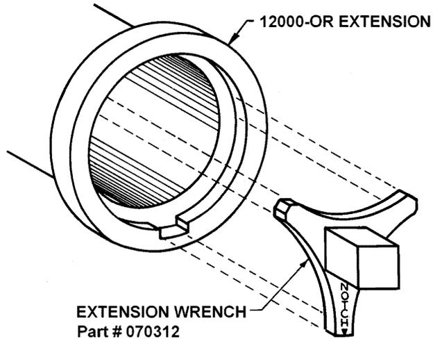
Use 12000-OR wrench to apply forward pressure as you thread extension into 12000-OR faceplate.
