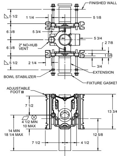
▲ FOR DIMENSION SHORTER THAN 5-1/2" (1" MIN) CUT EXTENSION. FOR LONGER EXTENSION (10-1/2" MAX) SPECIFY (-10)
