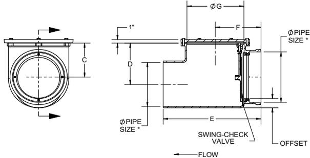
\* HUB & SPIGOT DIMENSIONS ARE IN ACCORDANCE WITH E.H.C.I. PIPE STANDARD.
