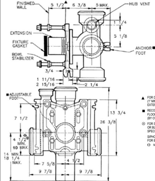
▲ FOR DIMENSION SHORTER THAN 5-1/2" (1" MIN) CUT EXTENSION. FOR LONGER EXTENSION (10-1/2" MAX) SPECIFY (-10)
