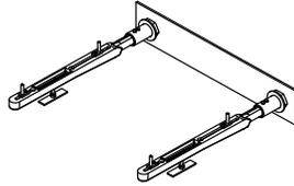
□: VARIABLE DIMENSION. DEPENDS ON FIXTURE. STANDARD ADJUSTABLE SLEEVE IS 4".
