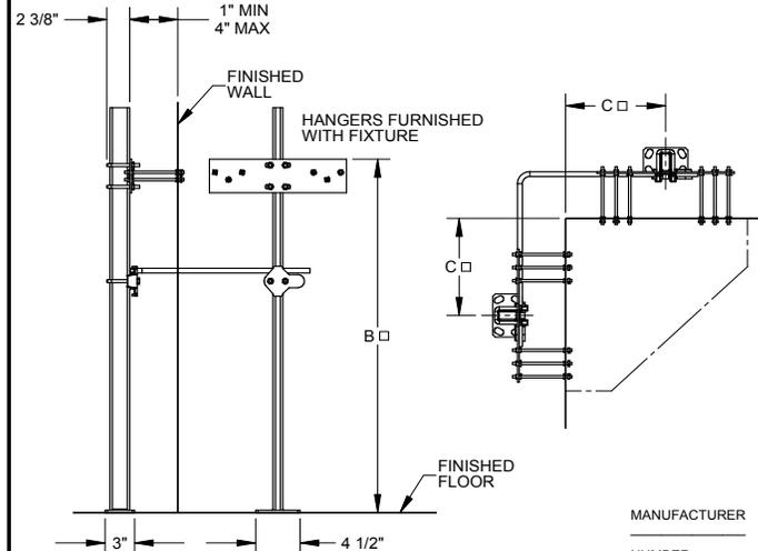
RECOMMEND ALL FEET BE SECURED TO FLOOR WITH 1/2" BOLTS AND ANCHORS BY OTHERS.
