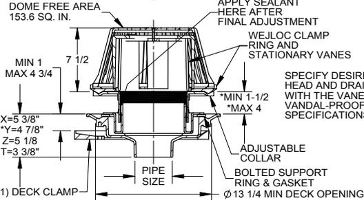
SPECIFY DESIRED FLOW RATE AND HEAD AND DRAIN CAN BE FURNISHED WITH THE VANES PRE-SET AND VANDAL-PROOFED TO THESE SPECIFICATIONS.
