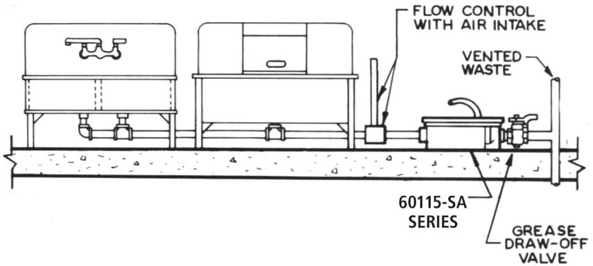
60115-SA Series Semi-Automatic shallow Interceptor installed on floor, servicing a double compartment sink and dishwasher.
