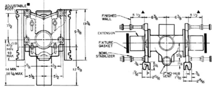
▲ FOR DIMENSION SHORTER THAN 5-1/2" (1" MIN) CUT EXTENSION. FOR LONGER EXTENSION (10-1/2" MAX) SPECIFY (-10)
