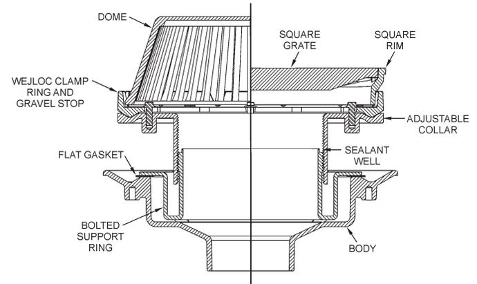
The adjustable integral top is mated to the body and support ring with a heavy machined thread which permits virtually unlimited top level adjustment to accommodate various deck thicknesses. The line contact between the threads provides positive circumferential support of the top at any adjusted elevation.
