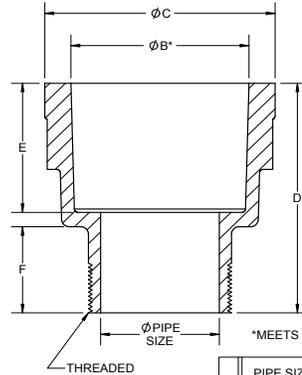
\* MEETS ASTM A-47 XH CAST IRON SOIL PIPE STANDARD
