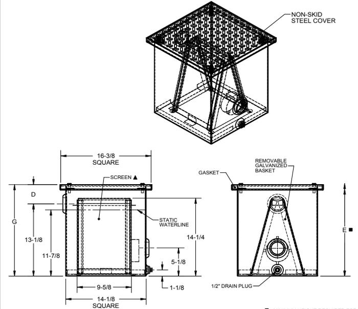
▲ REMOVABLE STAINLESS STEEL WIRE SCREEN - 40 x 40 MESH WITH .015\" OPENINGS
