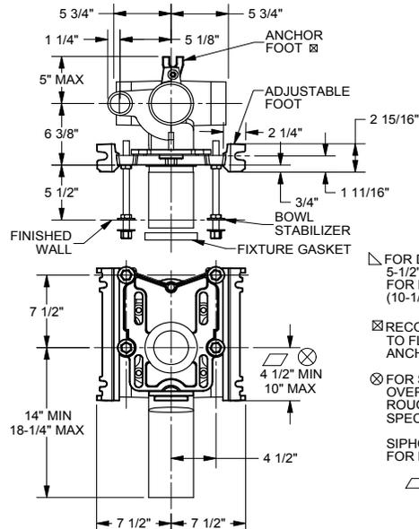
□ FOR DIMENSION SHORTER THAN 5-1/2" (1" MIN) CUT EXTENSION. FOR LONGER EXTENSION (10-1/2" MAX) SPECIFY (-10)
