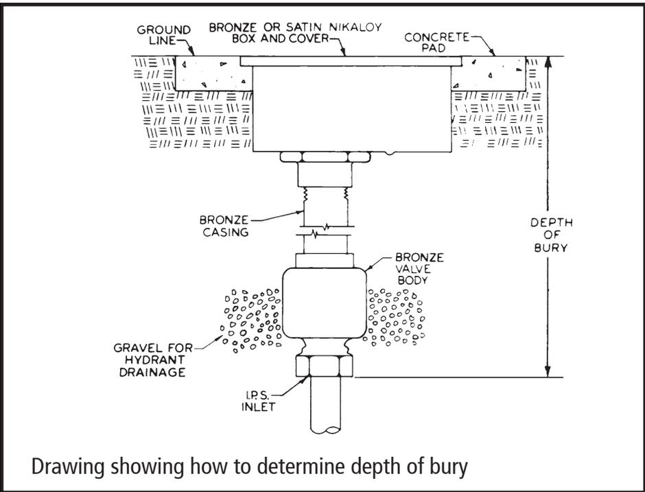
Drawing showing how to determine depth of bury
