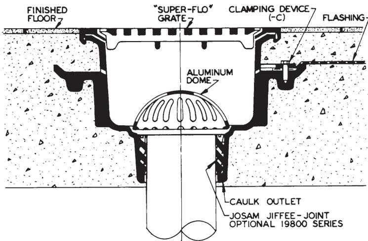
49320A-NB Series SUPER-FLO-SEPTOR® Floor Sink shown installed in a heavy-duty structural concrete finish floor.
