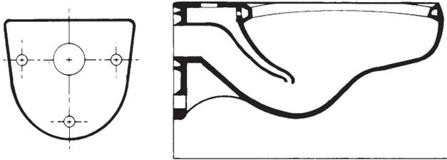
This type is particularly suited to heavy use applications such as public facilities in stadiums and terminals. The flushing action produced by the jet of water in the outlet passage is strong for rapid evacuation of the bowl. Fouling problems are minimal. However, because of the powerful flushing action, this type of closet is noisy to operate.
