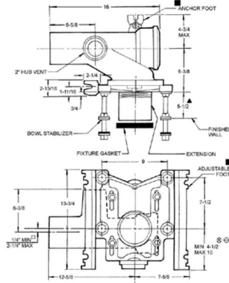
▲ FOR DIMENSION SHORTER THAN 5-1/2" (1" MIN) CUT EXTENSION. FOR LONGER EXTENSION (10-1/2" MAX) SPECIFY (-10)
