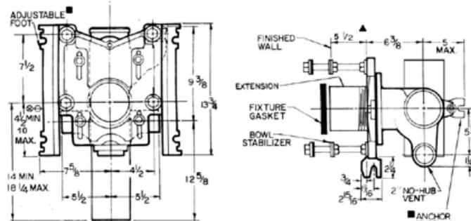
▲ FOR DIMENSION SHORTER THAN 5-1/2" (1" MIN) CUT EXTENSION. FOR LONGER EXTENSION (10-1/2" MAX) SPECIFY (+10)
