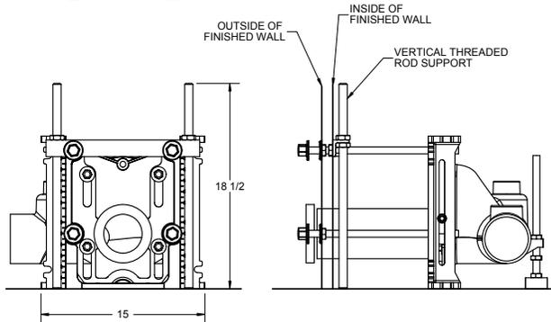
RECOMMEND CONCRETE ANCHORS WITH 750 LBS. PULL-OUT FORCE EACH.
