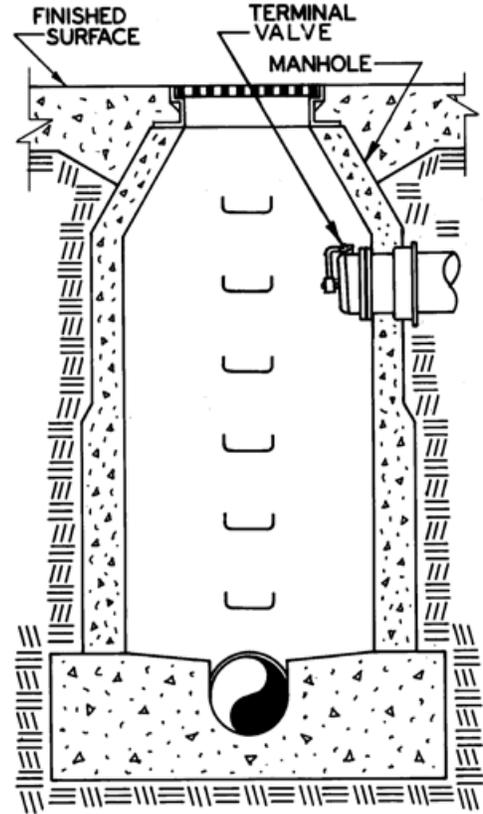
67800 Series swing-check Backwater Valve shown installed in a manhole terminal.
