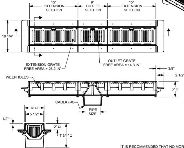
IT IS RECOMMENDED THAT NO MORE THAN EIGHT (8) EXTENSION SECTIONS BE USED WITH ONE (1) OUTLET SECTION
