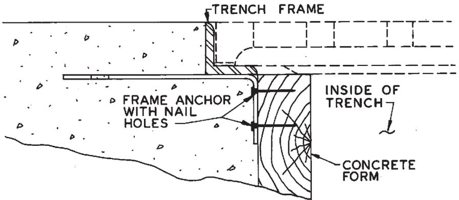
76700 Trench Frame and Grate for poured-in-place trench drains.
