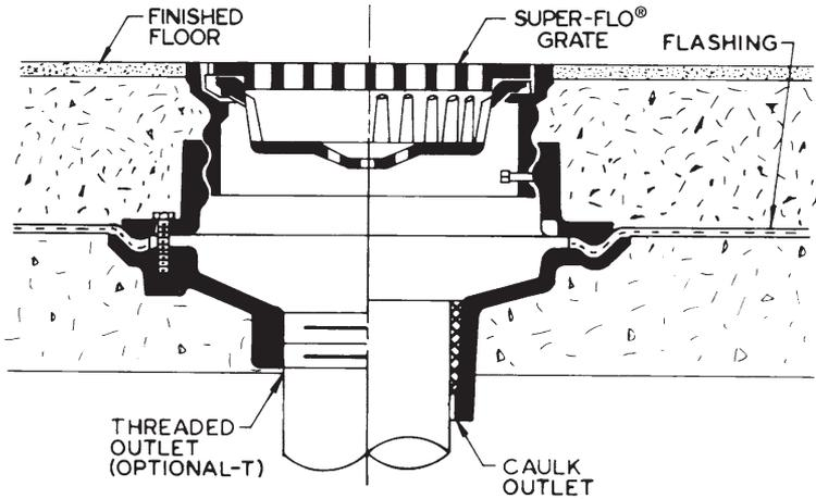
32100-AE-81 Series SUPER-FLO® Floor Drain shown installed in a poured concrete floor with floor finish. LEVELZE® Adjustable Collar provides vertical adjustment, facilitating installation and forming a perfect surface between top of drain and floor finish.
