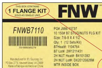
**NOTE:** Figure B7K flange kits are tagged with a yellow label to indicate that this is a complete set for one flange connection. The yellow tag differentiates these kits from the white tag boxes used for our bulk sold figure B7 stud/nuts.
