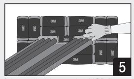
Seal any gaps with a minimum 25mm depth of  $3M^{\mbox{\tiny M}}$  Fire Barrier Moldable Putty MP+.
