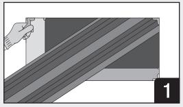
Apply a 12mm diameter bead of 3M™ Fire Barrier Moldable Putty Stix MP+ into each corner of the opening, extending a distance of minimum 30mm along each edge.
