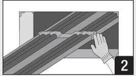
Firestop through-penetrants appropriately as per system specifications (e.g., wrap strips around non-metallic pipes, putty around cables).
