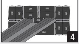
Fill the opening with additional rows of compressed, tightly butted pillows. Tightly pack the pillows around the through-penetrants, using a combination of available sizes to get the best seal.
