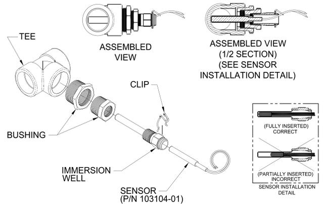
**Figure 48: Recommended “Immersion” type Header Sensor Installation Detail**
