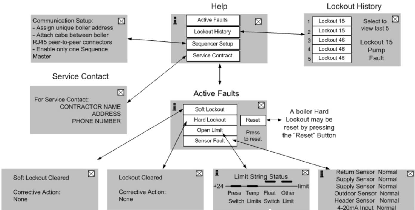
The "Help" screen provides access to active faults, lockout history, the service contact and the boiler reset button. The "Help" screen is accessed from the "Home" screen.
