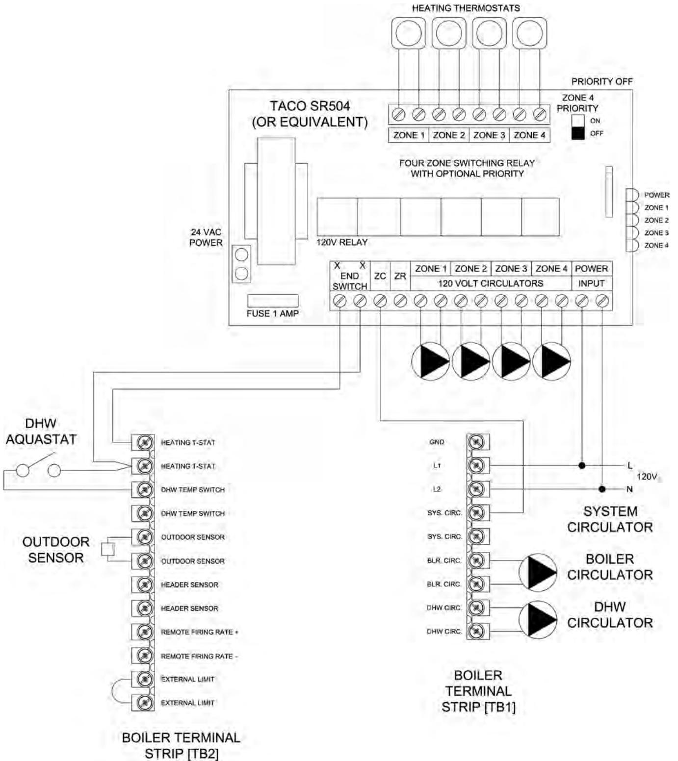
**\*\*\*USE SAME POWER SOURCE FOR ALL CONTROLS AND ENSURE POLARITY TO ALL CONTROL DEVICES IS CORRECT**
