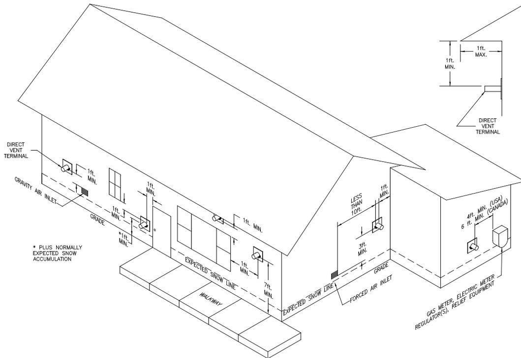
**Figure 3: Location of Vent Terminal Relative to Windows, Doors, Grades, Overhangs, Meters and Forced Air Inlets (Concentric Terminal Shown - Two-Pipe System Vent Terminal to be installed in same location - Two-Pipe System Air Intake Terminal Not Shown)**
