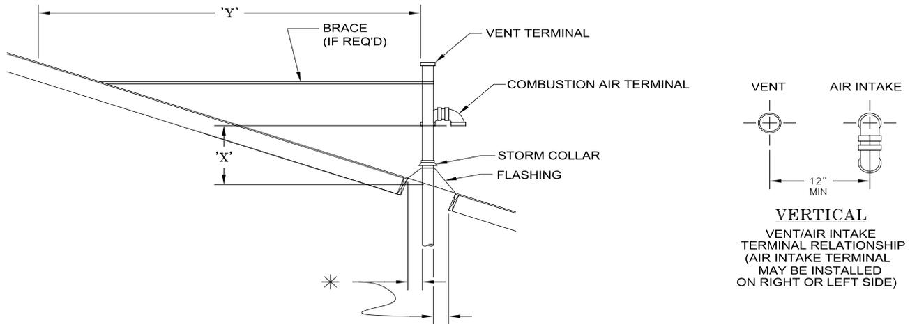
\* VENT PIPE MINIMUM CLEARANCE TO COMBUSTIBLE MATERIAL IS ONE (1) INCH. COMBUSTION AIR PIPE MINIMUM CLEARANCE TO COMBUSTIBLE MATERIAL IS ZERO (0) INCHES.
