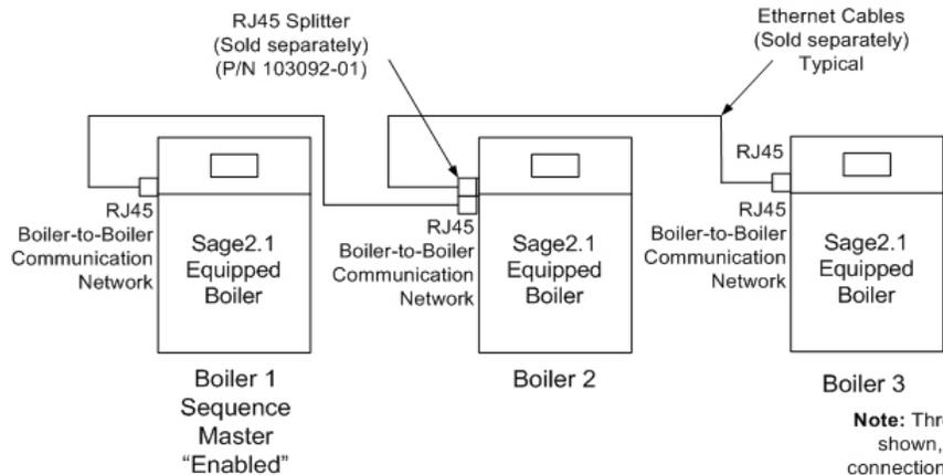
**Note:** Three boilers shown, typical connections for up to eight boilers
