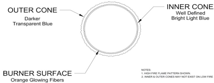
Figure 52: Burner Flame
