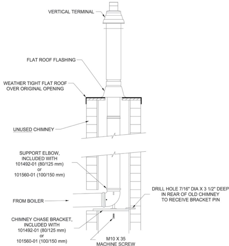
**Figure 28: Chimney Chase Installation**
