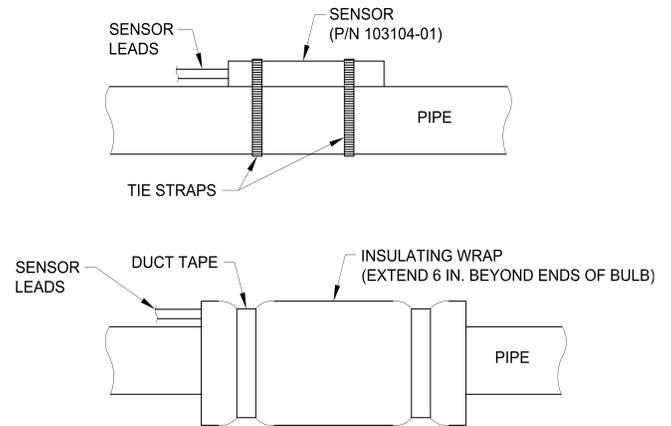
**Figure 49: Alternate “Strap-on” type Header Sensor Installation Detail**
