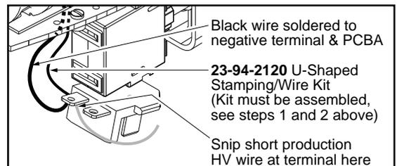
**SERVICE WIRING-** When installing a service replacement U-Shaped Stamping/Wire Kit (23-94-2120) it is recommended to snip old HV wire system at battery terminal. Remove and discard that short wire, closed end connector and longer wire with U-Shaped Stamping. Follow instructions to install new wire kit.
