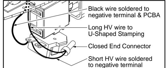
**PRODUCTION WIRING-** For ease in production, the Electronics Assembly (Switch, Stator, PCBA and Battery Terminal Block) has a short HV wire pre-soldered to the negative terminal. During production a longer HV wire (with a U-Shaped Stamping) is joined to short wire with an closed end connector.
