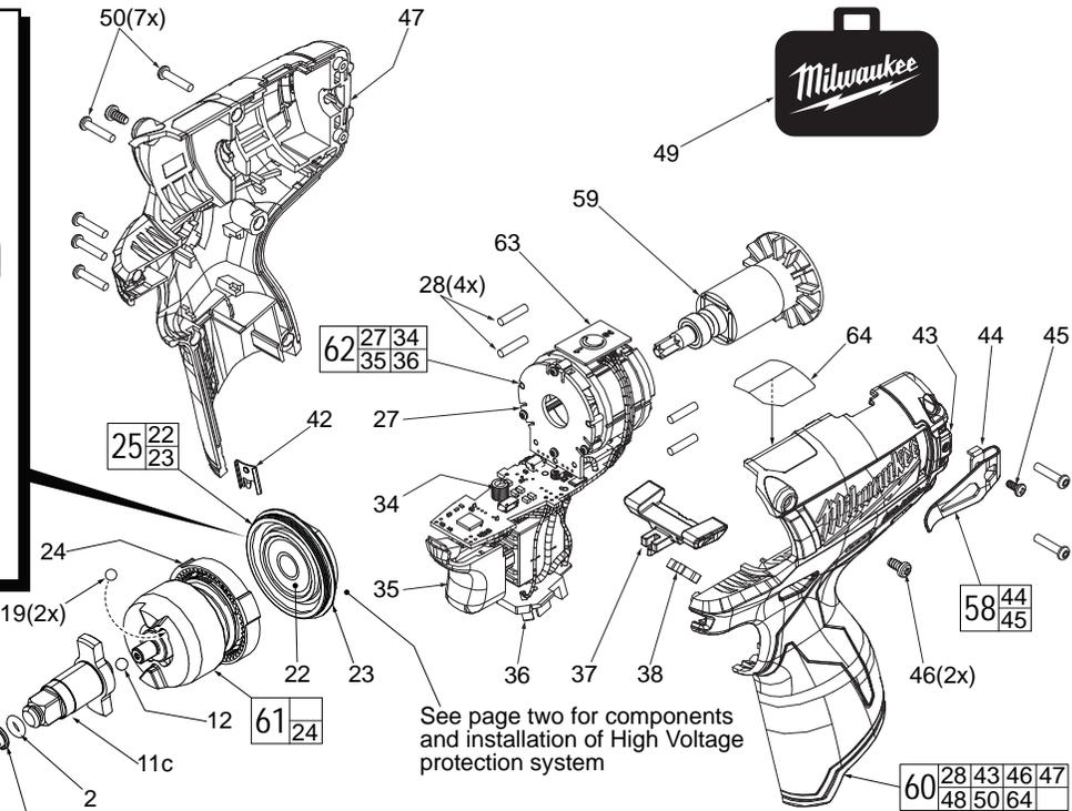
See page two for components and installation of High Voltage protection system
