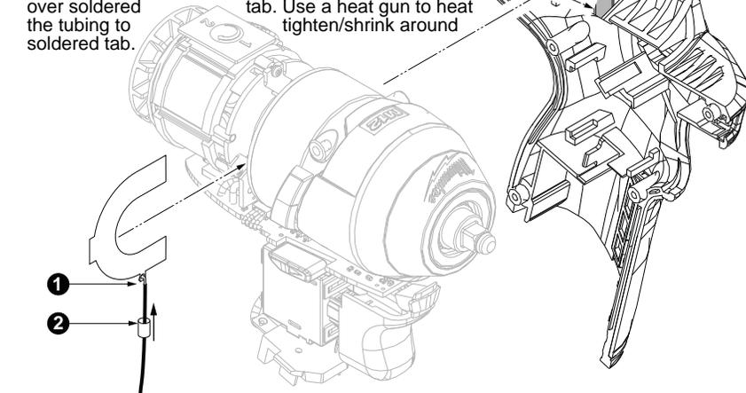
Route wire around PCBA and fwd./rev. shuttle (See below). Solder this end of wire to rear left terminal on battery connector block.
