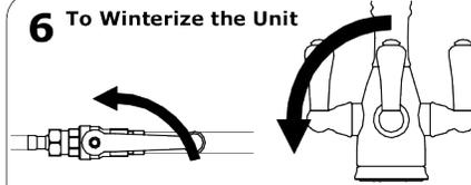
Shut off mains supply. A stop valve was supplied with the system for this purpose, and will be located on the adjacent pipe work.
