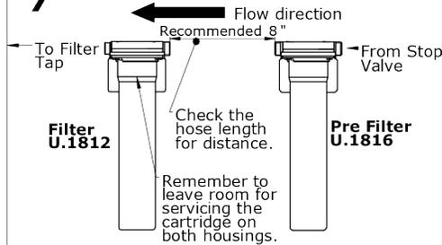
If installing a Pre-filter follow steps 1-3 for the second bracket taking into account the hose length supplied from the Pre-filter to the filter.
