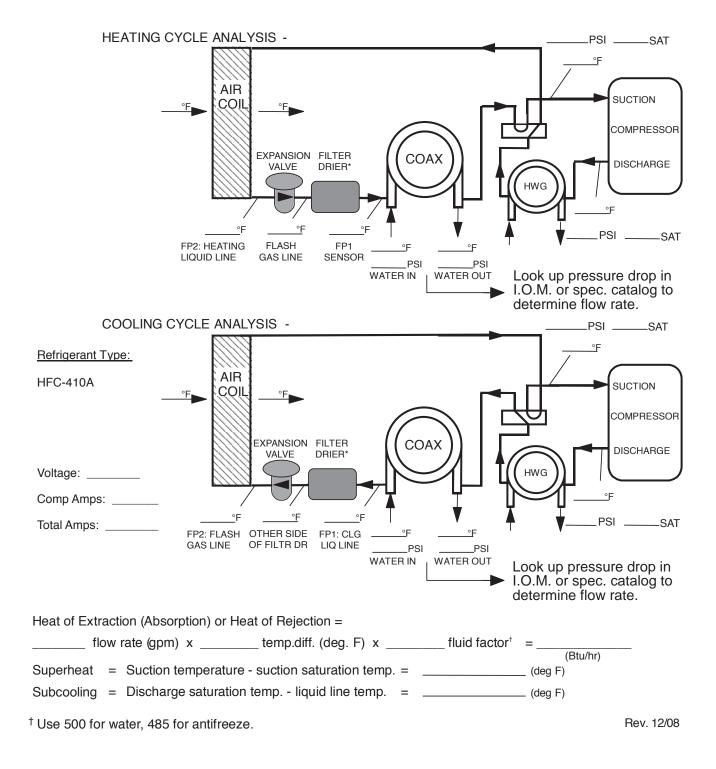
Note: Never connect refrigerant gauges during startup procedures. Conduct water-side analysis using P/T ports to determine water flow and temperature difference. If water-side analysis shows poor performance, refrigerant troubleshooting may be required. Connect refrigerant gauges as a last resort.
