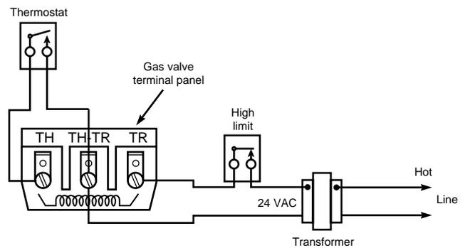
Figure 4. Wiring for 36C03 (24 Volt)
