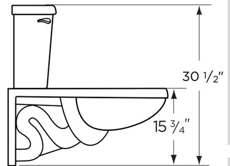
THIS FIXTURE QUALIFIES ACCORDING TO ASME TEST PROCEDURES AS A HIGH EFFICIENCY WATER CLOSET WITH AN AVERAGE CONSUMPTION OF 1.28 gpf (4.8 Lpf) OR LESS.
