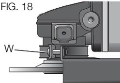
**⚠CAUTION:** Matching diameter backing flange and threaded locking flange (included with tool) must be used for Type 1 and Type 41 cutting wheels.
