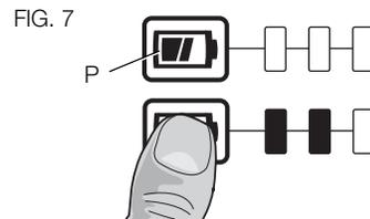
**NOTE:** The fuel gauge is only an indication of the charge left on the battery pack. It does not indicate tool functionality and is subject to variation based on product components, temperature and end-user application.
