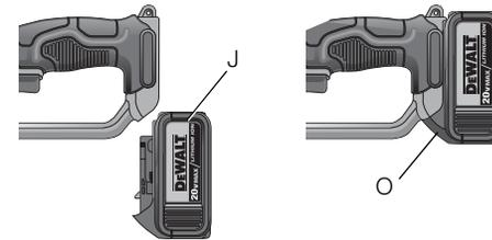
To install the battery pack (J) into the tool handle, align the battery pack with the rails inside the tool's handle and slide it into the handle
