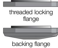
**NOTE:** If the wheel spins after the threaded locking flange is tightened, check the orientation of the threaded locking flange. If a thin wheel is installed with the pilot on the locking flange against the wheel, it will spin because the height of the pilot prevents the locking flange from holding the wheel.
