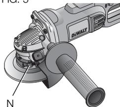
**NOTE:** The guard is pre-adjusted to the diameter of the gear case hub at the factory. If, after a period of time, the guard becomes loose, tighten the adjusting screw (N) with clamp lever in the closed position with guard installed on the tool.
