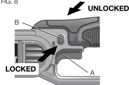
To unlock the trigger switch, press the lock-off button. When the lock-off button is depressed to the unlock icon, the unit is unlocked. The lock-off button is colored **red** to indicate when the switch is in its **unlocked** position.
