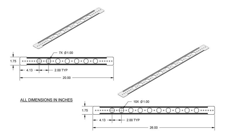
The LOCKRITE™ #601-20 and #601-26 are 20 gage galvanized steel brackets designed exclusively to support CPVC piping. Rolled edges provide added strength. Works exclusively with our glueable HOLDRITE® #604 (1/2") or #605 (3/4") inserts. Inserts snaps into bracket.
