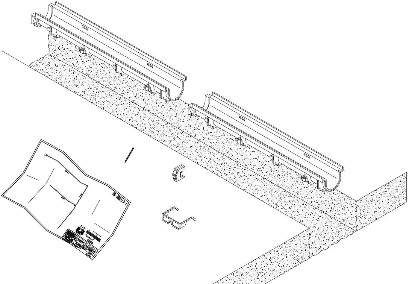
Upon completion of the trench excavation, the channels should be placed in order alongside the excavation and according to the job layout. Grates are not installed at this time.
