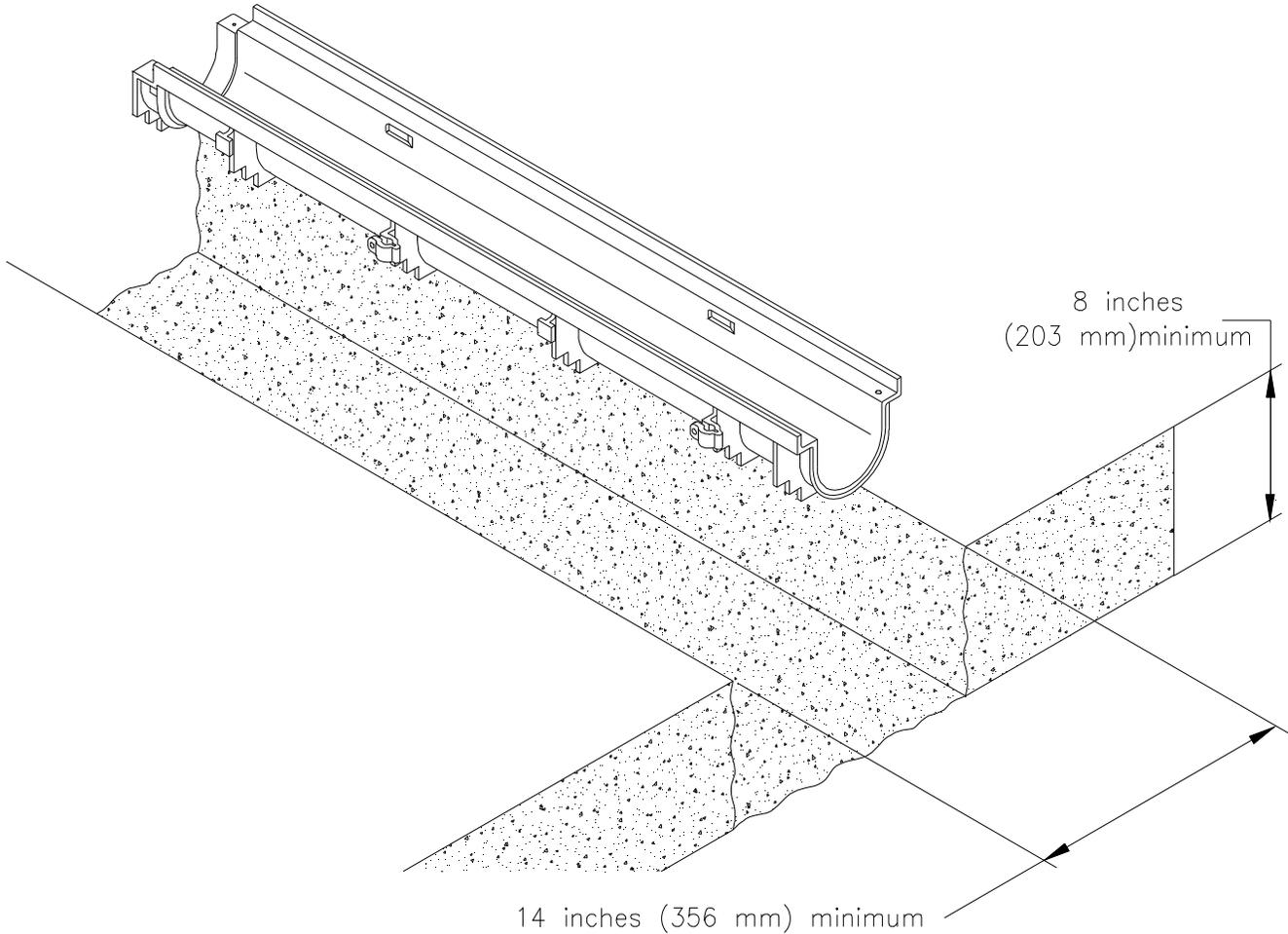
Trench excavation must be 4 inches greater than the trench depth and a minimum width of 14 inches. Soft and/or shifting soil substrates may cause cracking of the concrete and consequent movement of the trench. It is critical that the concrete be poured on an adequate foundation.
