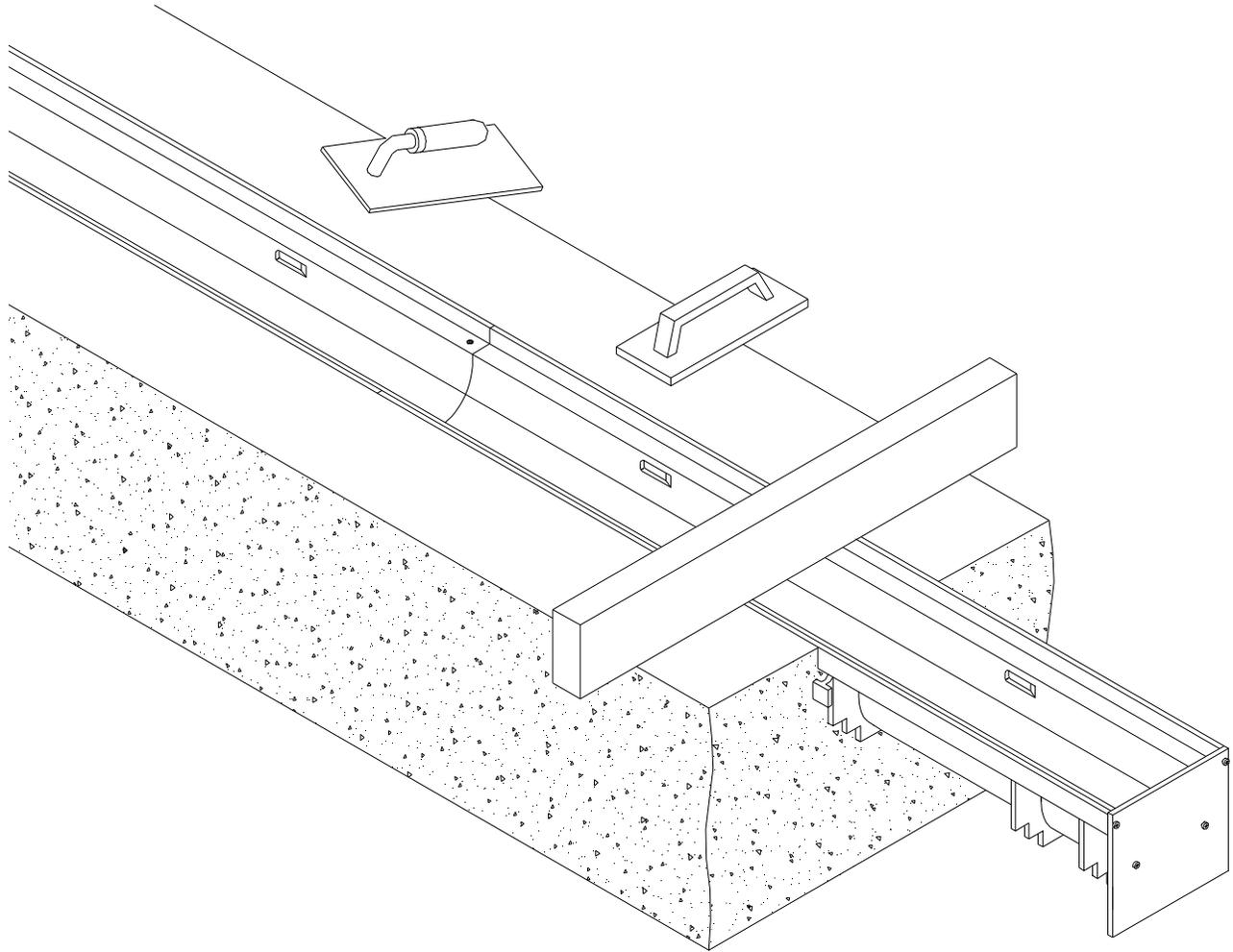
It is necessary to install a 108mm wide spacer (supplied by others) in the grate section of the trench to maintain the width during the concrete pour.
