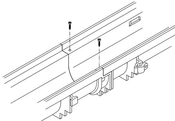
Assembling the trench run is easy using 'Flo-thru's' mechanical interlocking joints. Simply align the two mating ends of the trench sections and fasten with the hardware fasteners provided. A silicone caulk, or a construction adhesive, such as Liquid Nails, is recommended to be used at each joint as a sealer.
