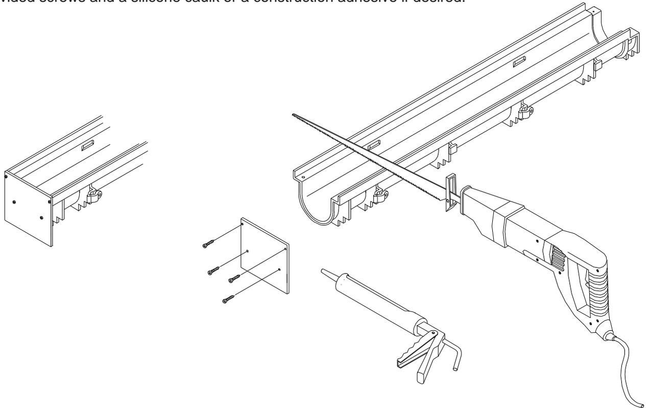
A bottom outlet is attached to the bottom side of the trench drain with provided screws and a silicone caulk or a construction adhesive if desired as shown below. A hole saw can be used to cut the appropriate size hole through the bottom of the trench.
