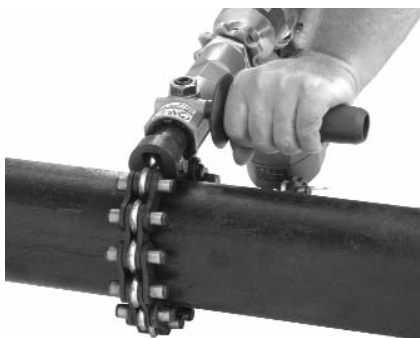
Figure 5 – Operating the Powered Soil Pipe Cutter – Using Impact Tool
