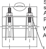
Stainless Steel Nuts and Studs - Type 304 stainless steel studs per ASTM A193 and A194. Heavy hex nuts are coated to prevent galling.
