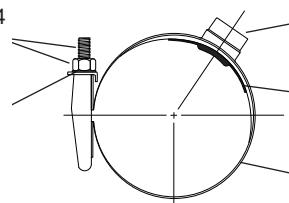
Stainless Taps - Type 304 stainless steel TIG welded to shell. Available with AWWA, FIP or BSP threads 1/2" thru 2".
