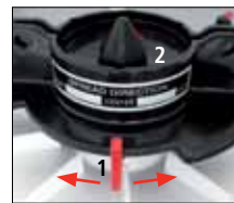
Adjustable distribution direction (1), agitator (2)
