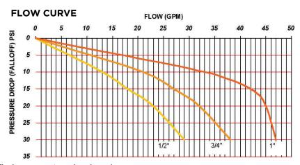
\*Falloff is the difference between the PRV's set pressure and the flowing pressure at any given demand Pressure Differential is the difference between the inlet supply pressure and the adjusted outlet pressure. Pressure Falloff is the reduction in downstream pressure from the static (set) pressure as the flow increases through the valve.
