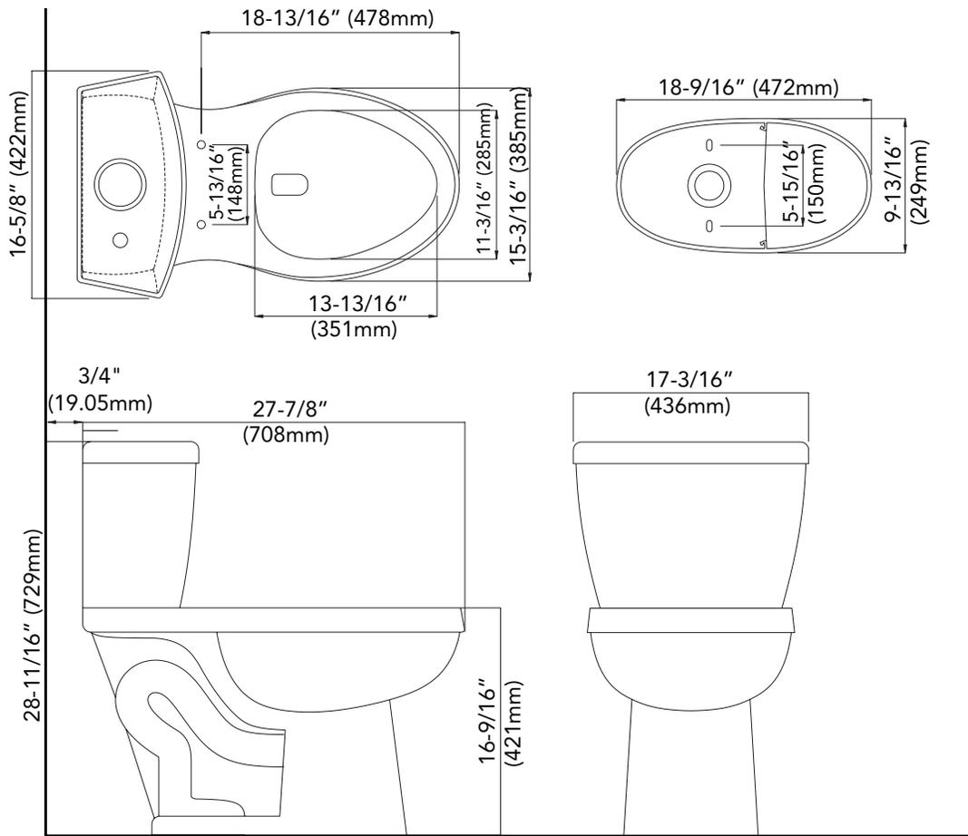
Note: All dimensions and specifications are nominal and may vary: Dimensions of 8" and greater have a tolerances of +3%. Dimensions less than 8" have a tolerances of +5%.
