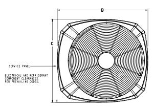
TOP DISCHARGE AREA SHOULD BE UNRESTRICTED FOR AT LEAST 1524 (5 FEET) ABOVE UNIT. UNIT SHOULD BE PLACED SO ROOF RUN-OFF WATER DOES NOT POUR DIFFCTLY ON UNIT. AND SHOULD BE AT LEAST 305 (12") FROM WALL AND LEAST AND SHOULD SURROUNDING SHRUBBERY ON TWO SIDES. OTHER TWO SIDES UNRESTRICTED.
