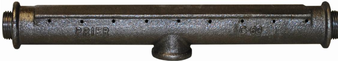
The C-69 Cast Iron Burner Bar is the original burner bar with ash shields to prevent clogging of the gas ports. The tee style design has three 1/2" I.P.S. tappings for gas service from bottom or either side. The burner bar is shipped with two plugs for the unused ports
