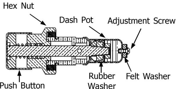
**To Install:** Remove old flush valve assembly and make sure the valve is free from debris or defects. Install flush valve into the assembly and tighten. Tighten to 90 in/lbs pressure.
