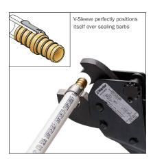
2. Compress tool perpendicular to tube - Compress only once. Remove any defective connections. Use a gauge to assure a proper joint.
