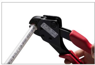
4. Compress tool perpendicular to tube. Compress only once. Remove defective connections. Use a gauge to assure a proper joint. Test all completed joints.
