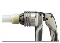
3. Using expander tool, expand sleeve fully. Repeat expansions, rotating expander 1/8-turn between expansions.
