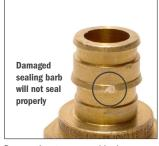
Damaged, cut or grooved barb on fitting.
