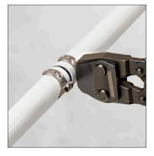
2. Close clamp ear with ratchet pincer tool. Tool will not release until clamp is fully closed. Remove any defective connections.
