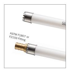
1. Cut tube at 90-degrees. Install V-Sleeve onto OD of tube with notched side towards tube end. Install fitting fully into tube. Visually confirm tube is fully inserted through notches.
