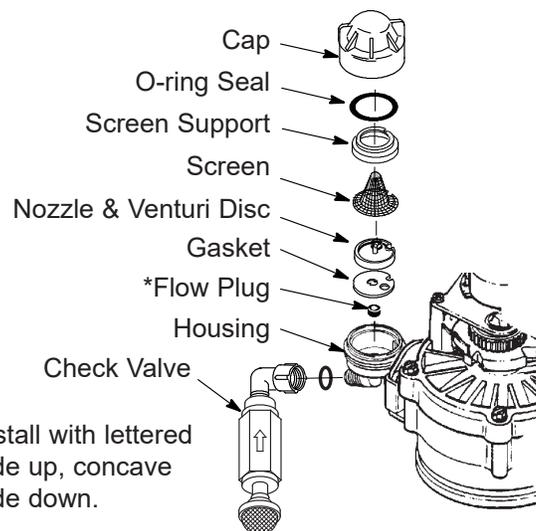
**IMPORTANT:** Be sure small hole in the gasket is centered directly over the small hole in the nozzle & venturi housing. Be sure the numbers are facing up
