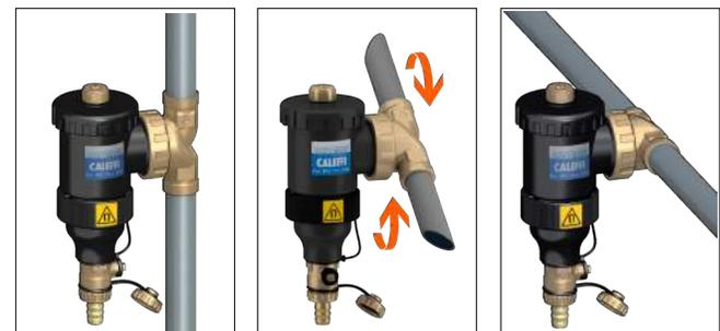
The special coupling between the locking nut and the mounting base allows the DIRTMAG® dirt separator to be rotated for installation to either vertical or horizontal pipes, while maintaining the same operating performance.
