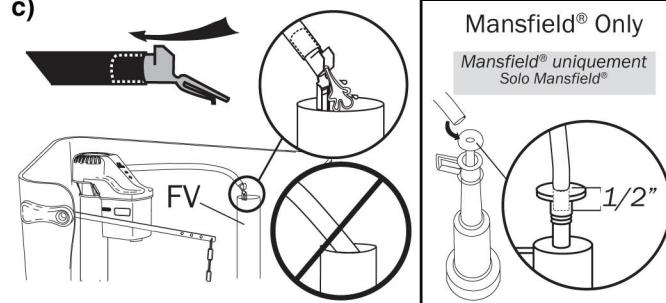
Attach tube to flush valve (FV) with metal clip so
