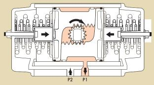
For clockwise output, the volume between the pistons is exhausted to P1, causing the springs to force the pistons together. Air is admitted through P2 as pistons move together.
