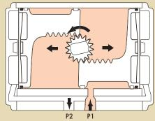
For counterclockwise output, apply pressure to P1, which forces the pistons apart. The linear travel of the pistons is converted to a rotation of the output shaft by rack to pinion connection. The volume outside each piston is exhausted at P2.
