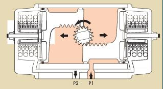
For counterclockwise output, apply pressure to P1, which forces the pistons apart and compresses the springs. The linear travel of the pistons is converted to a rotation of the drive shaft by rack to pinion connection. The volume outside each piston is exhausted at P2
